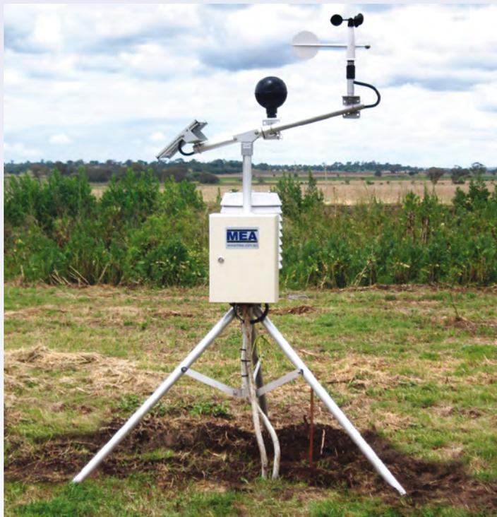
Measurement of the Heat Load Index for livestock can be calculated on an MEA weather station especially fitted with a Black Globe Temperature Sensor. This blackened copper sphere has a thermistor temperature sensor at its centre, and provides an output via an algorithm used by the feedlot industry to measure solar stress on their cattle.
