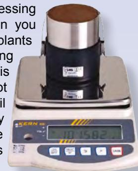
If you don't have a soils lab – and very few of us do – then there is now a simple way of figuring this out, using a Hyprop© apparatus (JMS, Germany) to determine pF-curves and the unsaturated hydraulic conductivity of soil samples from standard 250 ml soil sampling rings. Again, call Sonja at MEA for more information.
